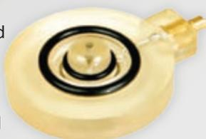
The electrode disc comprises a central platinum cathode and a concentric silver anode. Preparation of the electrode includes the addition of electrolyte and the application of a thin oxygen permeable P.T.F.E. membrane to the electrode dome.
